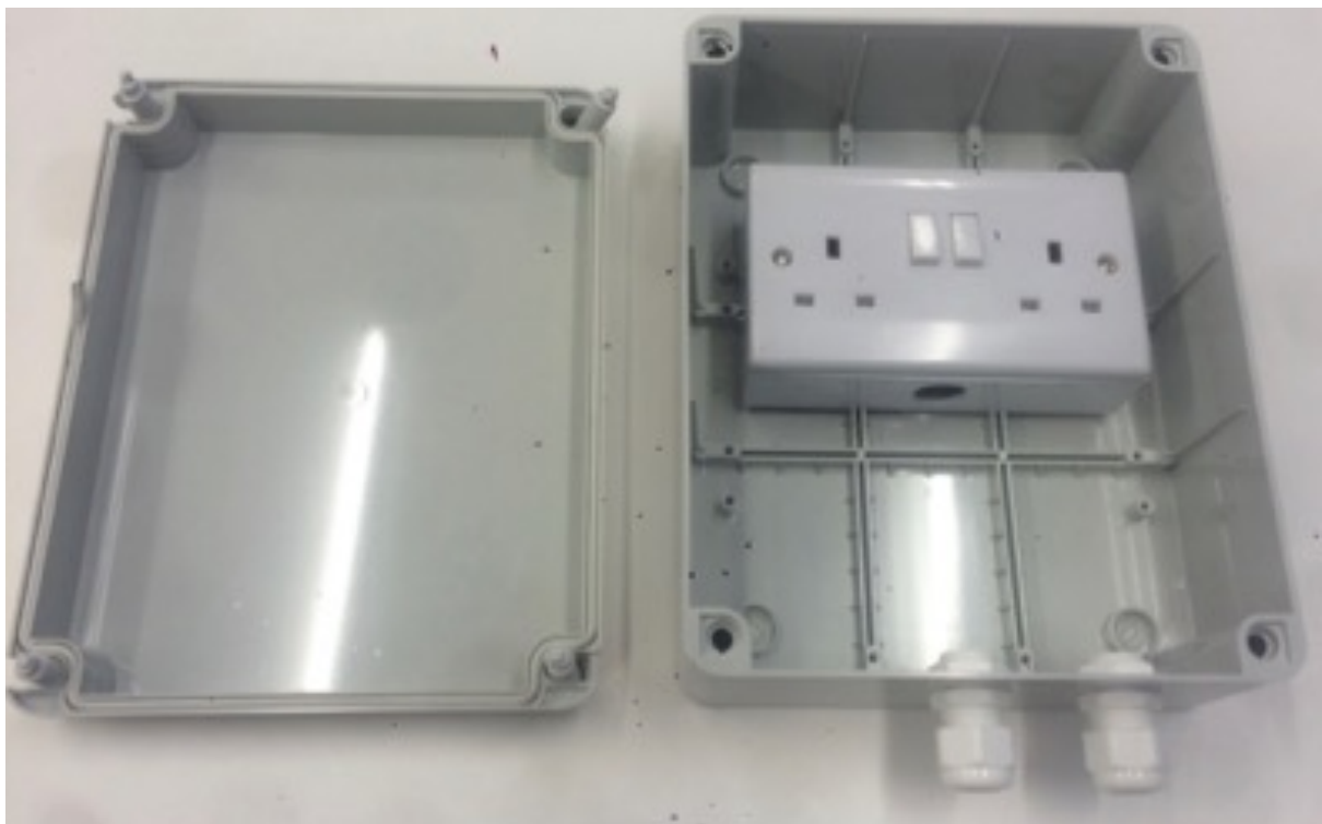
Example of completed box Internal dim. LxHxD (mm) 240x190x90mm.
